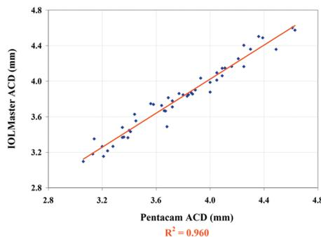
Fig. 3—Scattergram of the anterior chamber depth (ACD) measurements of the IOLMaster plotted against those measured by the Pentacam.
